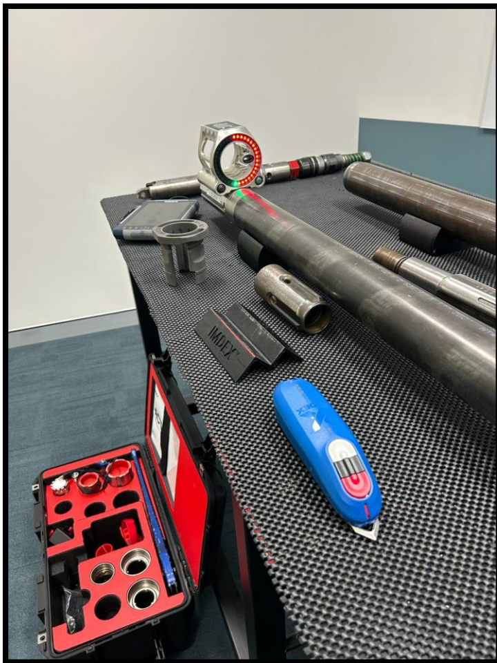
The entire kit. The Smart Jig is sitting in docking groove on the ACTx attached to the core barrel. A tough tablet is paired to the devices and a sleeve for the Smart Jig for different core sizes sits in front of it. A piece of bent metal with an IMDEX logo sits behind the latest version of the blue iQ-Logger. The red box is the Smart Jig – ACTx kit with couplings etc.
