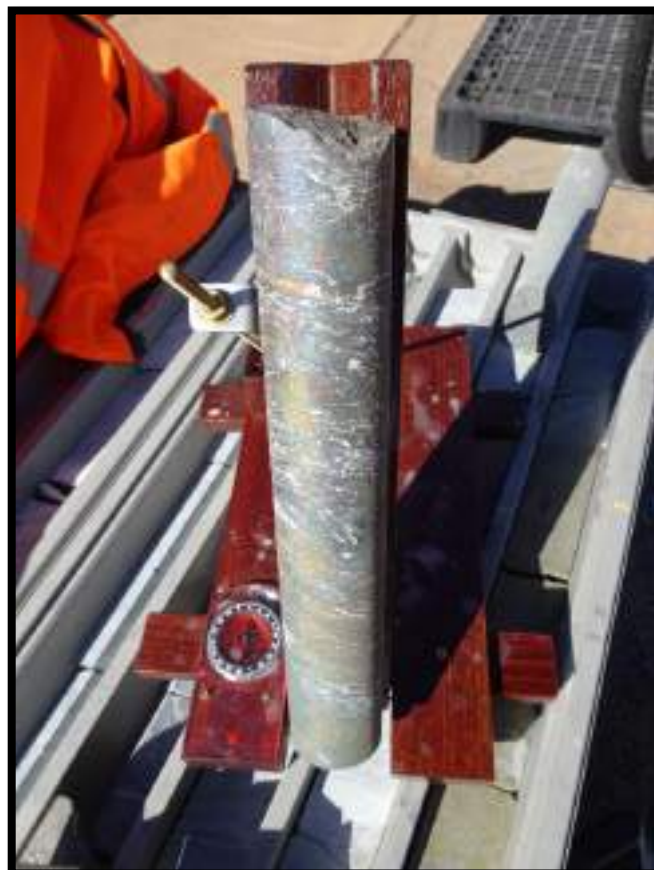
Example of a core orienting frame with the horrible threaded rod adjustment design
