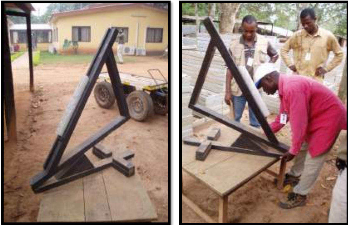
Core frame with angle adjustment via movement of a wooden wedge.
