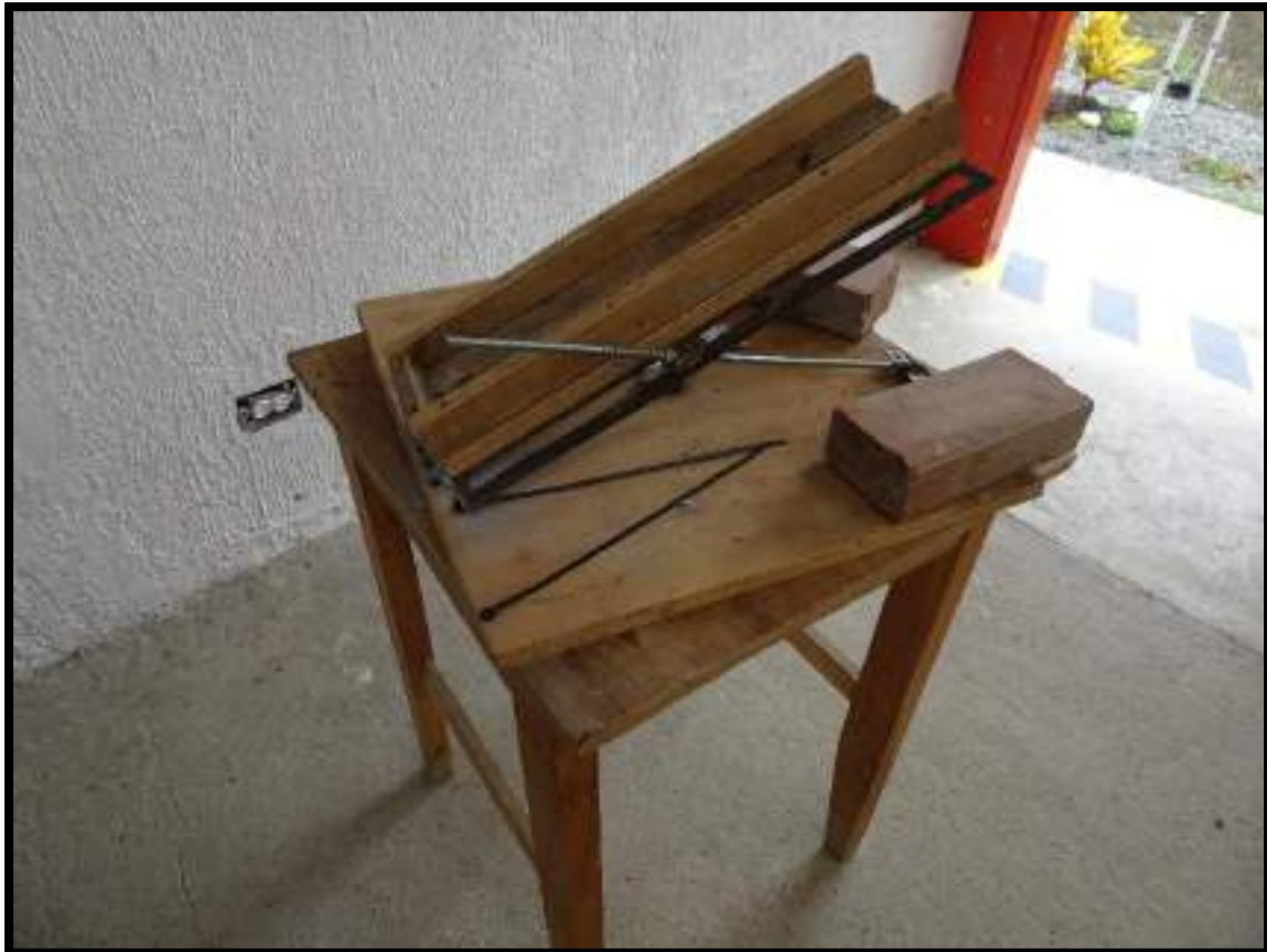
The most annoying angle adjustment mechanism around – the threaded rod with a nut that has to be tediously screwed up and down.
