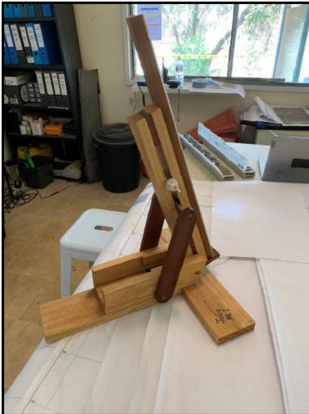
The Julie MK1 core orientation frame. All timber and a very useful prototype built by one of the geologists working on the project. Hard to see the orientation line though, due to the cradle being solid and having the wooden support for adjusting the angle behind it.
